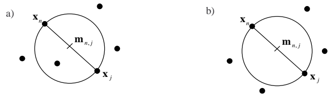
FIG. 6: Illustration of nearest neighborhood search by DT approach a) \mathbf{x}_j and \mathbf{x}_n are not near neighbors. b) \mathbf{x}_j and \mathbf{x}_n are near neighbors
